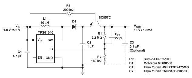
Figure 18. LCD Bias Supply With Load Disconnect
