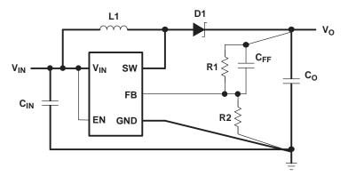
Figure 15. Layout Diagram
